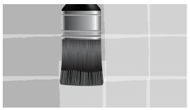
pattern the second coat should be applied in left to right patterns. It is recommended to make sure that all the concrete that has been casted internally and externally is coated properly with **Water Guard Crysta Coat 101** (For further application guidance, please refer to the product datasheet).
