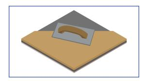
Prepared surfaces should be primed using **Ressi EPO Primer**. The primer should be brushed into the substrate using a stiff brush or roller & allowed to become tacky (10-20 mins) before the application of **Ressi EPO Tough Might**. The primer should be allowed to dry. If the primer has dried, additional coat of the primer should be applied & allowed to become tacky.
