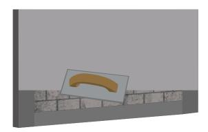
Adding **Ressi SBR 5850** & **Silmix** in the plaster Mix: A plaster comprising of a good ratio can also be applied over the wall area. It is recommended to add **Ressi SBR 5850** & **Silmix** into the plaster mix. The recommended dosage of **Ressi SBR 5850** & **Silmix** is 1 Ltr each to be added with the mix of every 50 KG bag of cement. Once the plaster has been applied & cured properly. Subsequent treatment can be done over the wall.
