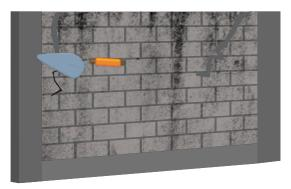
Assessment of the surface: if upon inspection irregularities in the surface of the concrete or masonry are found, like dampness or salt bursts, they should be addressed. For guidance on how to address salt bursts & dampness, please refer to solution for addressing salt bursts using acid itching. In case there is an issue of dampness of the area, it should be addressed using a recommended system by Ressichem.
