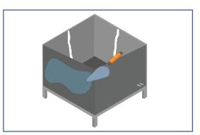
proper bonding between the pipe and the crystalline plugging material. The same treatment can also be repeated from the exterior side of the overhead tank.
