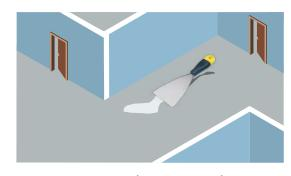
putty like paste of **Ressi EPO Crack Fill** material so that it can easily be applied with a scrapper.
