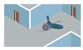
Once the crack has been opened and proper surface has been prepared, the surface is ready to take in the subsequent crack filling of **Ressi EPO Crack Fill.**
