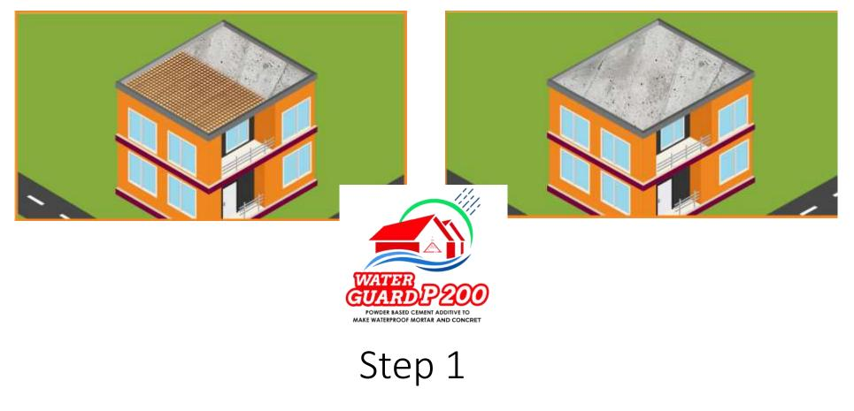
Pouring of the roof / balcony slab with the inclusion of Water Guard P 200.
