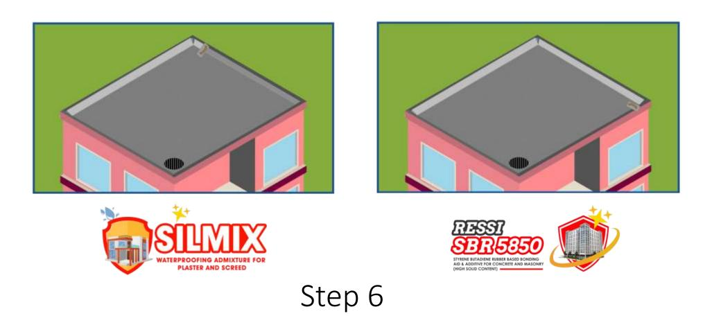
Making of chamfers with a cement sand mortar comprising of Ressi SBR 5850 and Silmix.
