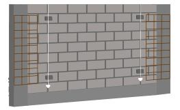
**STEP 2:** Application of **Ressi PlastoRend 120** directly on prepared masonry & concrete surface.
